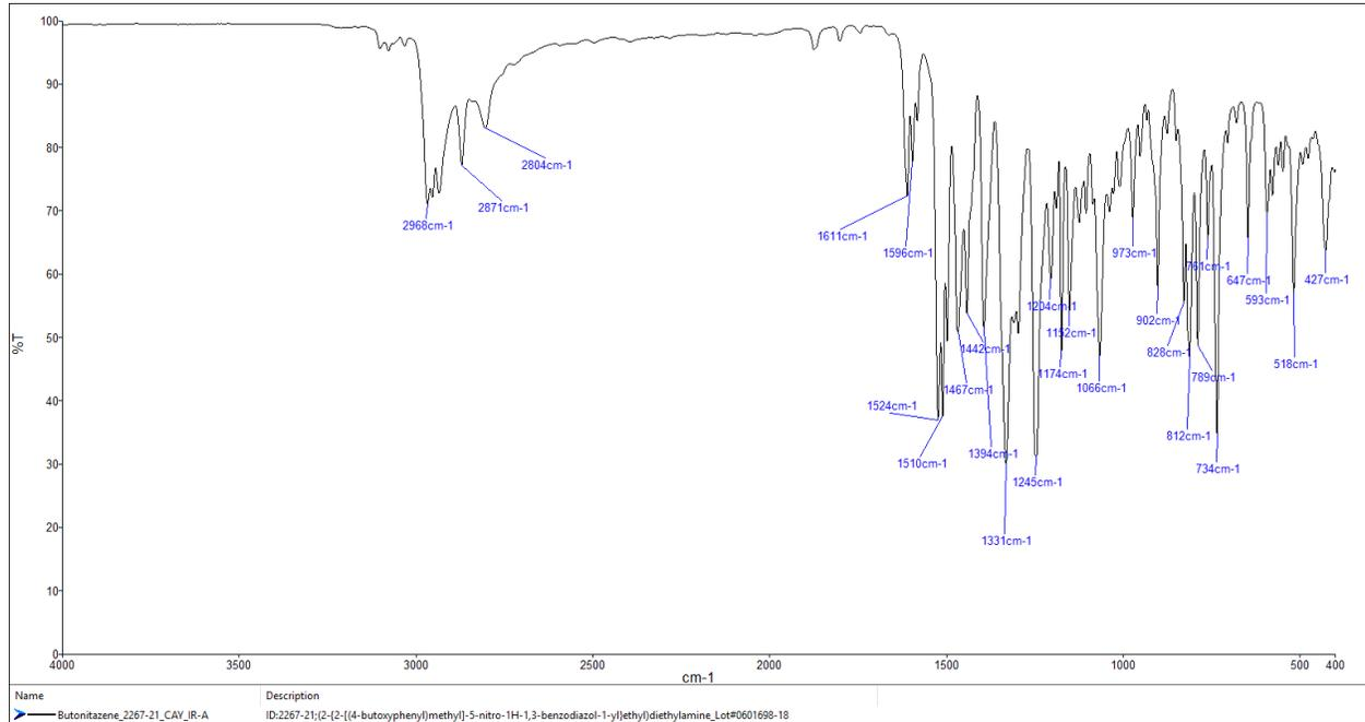
IR- (condensed (solid) phase – after chromatographic separation) - spectrum per base form
