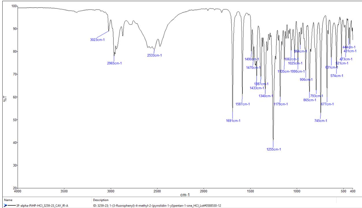
IR- (solid phase – after chromatographic separation) - spectrum per base form
